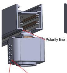
Continue to rotate until the latch snaps in place between the two track rails.
