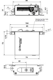
You can secure the controller by its side tabs to a flat mounting surface using screws or mount it on a TH35 DIN rail in your switch cabinet using the supplied DIN rail clin
