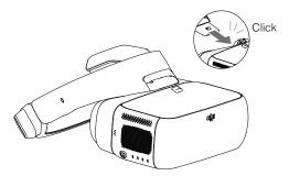
Press the Headband Buckle and move it in the opposite direction to release the Headband.
