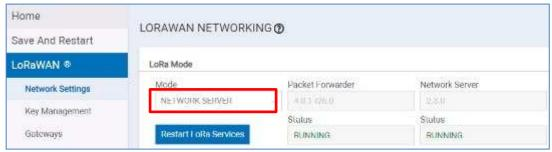
It is possible to set the Packet Forwarder mode to send the measurements of LoRa devices from a "slave" Gateway (Packet forwarder) to the "master" Gateway (Network Server) which must always be configured in fixed IP.
