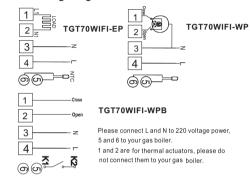
Remarks: please read wiring diagram carefully before connecting. If you connect it wrongly, there will be a short circuit. Your gas boiler board will be damaged!!!
