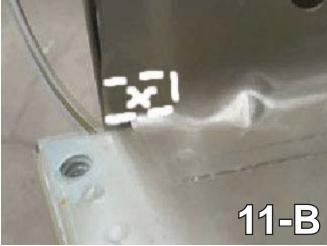
11. Cut the front webbing on the top edge of the frame and the 1/2" above the frame with the reciprocating saw. Bend the webbing toward the headlight area. Do this to both sides of the vehicle. This will open the area for the baseplate installation.
