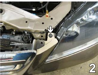
Remove one pushpin from the top edge of the fascia just inside of the headlight assembly. Do this to both sides of the vehicle.
