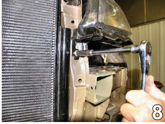
Using a 10MM socket, remove two metric bolts from the headlight assembly. Unplug and set the headlight assembly and metric bolts aside to be reinstalled later. Do this to both sides of the vehicle.
