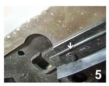
5. Remove the six pushpins from the lower edge of the fascia and the belly pan. Pull the fascia forward to remove. Set the pushpins and fascia aside carefully to be reinstalled later.
