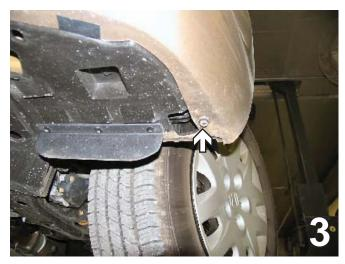
Using a 10MM socket remove one metric bolt from just forward of the front tire. Do this to both sides of the vehicle.
