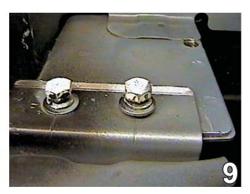
Using the 12MM socket, remove two metric bolts from the top of the metal bumper. Do this to both sides of the vehicle. Set the bolts aside to be reinstalled later.
