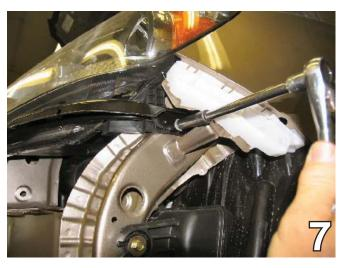
Using the 10MM socket, remove one metric bolt from the side of the headlight assembly.
