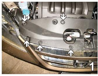
Remove the five push pins from the black plastic cover on the top side of the fascia. Do this to both sides of the vehicle. Lift cover up to remove. Set cover and pushpins aside to be reinstalled later.
