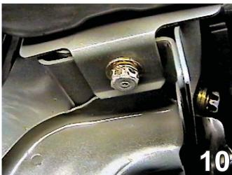
Remove the metric bolt from the bottom of the metal bumper with the 12MM socket. Pull the metal bumper forward to remove. The metal bumper will not be reinstalled.
