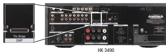
Figure 20 – The Bridge II Connection
