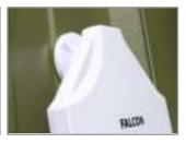
The high gain antenna is Omni-directional and can be placed anywhere. It is recommended that the antenna is placed as high as possible to avoid obstructions but not always necessary.
