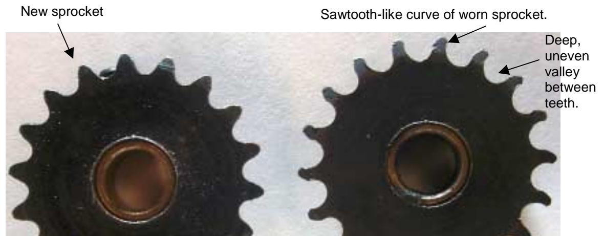
Fig: 8 A badly worn idler sprocket is shown at right above. A new sprocket is shown at left for comparison. Note the sawtooth-like directional curve of the worn sprocket's teeth. Also note the depth and uneven wear between the teeth. Sprockets showing this type of wear should be replaced.
