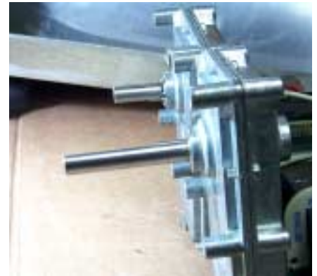
Fig: 5 The new motor (in front) has a longer drive shaft. Also the mounting points are not tapped. It is best to run the self-tapping bolts into the casing prior to placing the motor in place in the cabinet.
