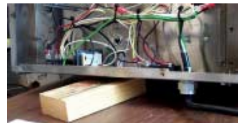
Fig 3 Rest the unit on a 2x4 or some similar object to avoid stressing the power cord.
