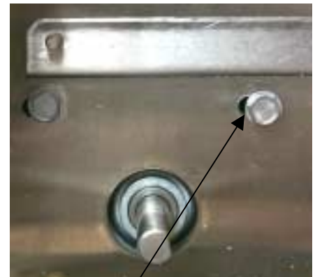
Fig: 6 Check the mounting slots before tightening the motor mounting bolts to ensure the motor is shifted toward the front of the toaster.
