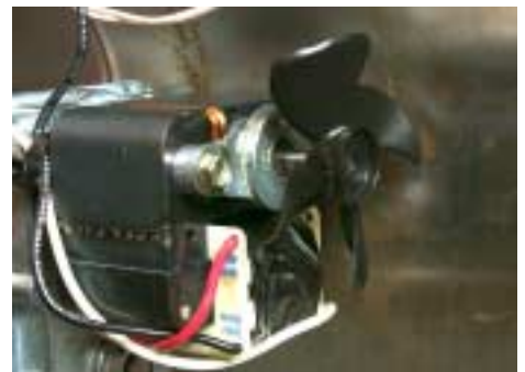
Fig: 9 The cooling fan on the rear of motor shaft should be flush with the end of the shaft as shown.
