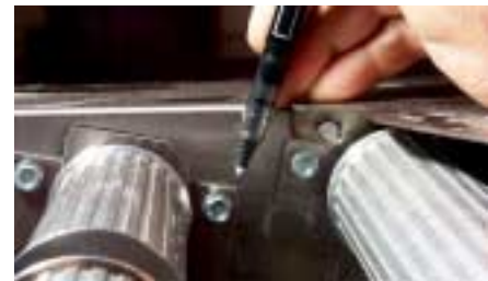
Fig: 17 This screw on the controller side of the front upper roller is removed to accommodate the placement of a crumb catcher.
