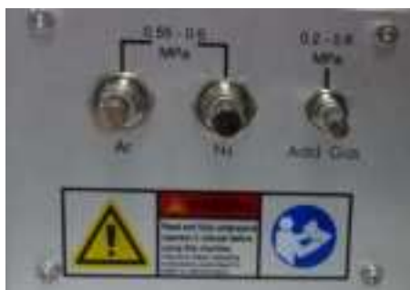
Figure 3-12. Connections on the instrument for gas supply
