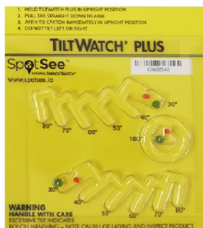
Figure 3-1. Shock and tilt indicators (green ball at 60° is the acceptable maximum tilt)
