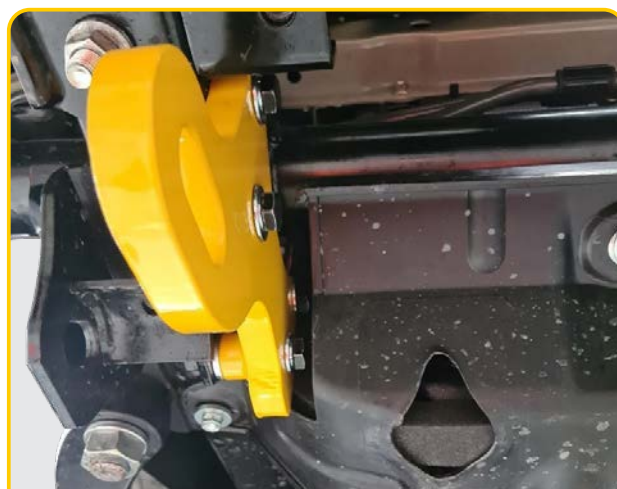
Figure 4 - Undertray in place after notching
