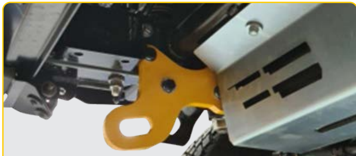
Figure 1 - Drivers side recovery point
