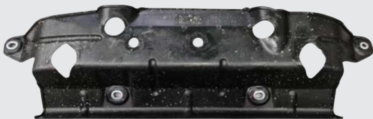
Figure 3 - Notching of plastic undertray
