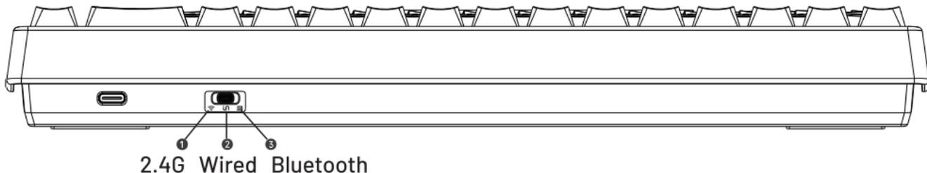
Note: The function of the lower cover switch of the wireless version is mode switching.
