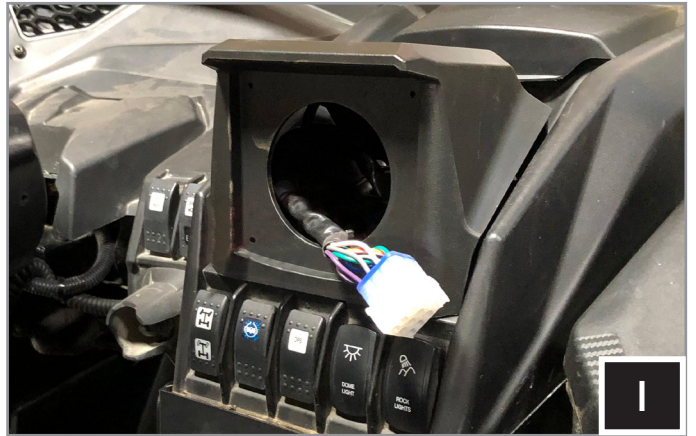
I. Place the DMR1 over the base plate with the harness routed out of it.
