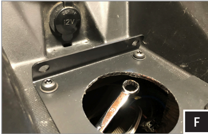
F. Place (4) M6 T30 screws and washers into each drilled hole. Fasten from the bottom a washer and M6 nut. Secure each screw with 10mm wrench and T30 torx driver.
