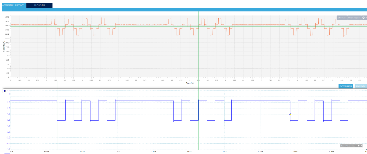
Figure 5. Example of STLINK-V3PWR trigger output with 2900 \mu\text{A} current threshold (current waveform in red with STM32CubeMonitor-Power, TGO signal in blue with PicoScope® software)
