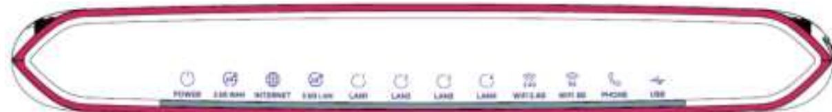
Figure 11 LED Indicators (EX5501-B0)
