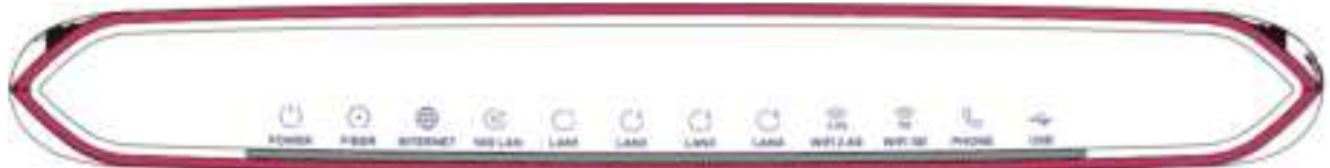
Figure 11 LED Indicators (EX5501-B0)
