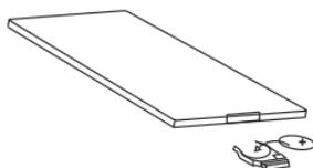
Fix the battery seat to the right position of the remote control
