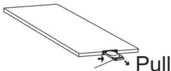
Put the battery to the right position (With the mark “2025” up side)
