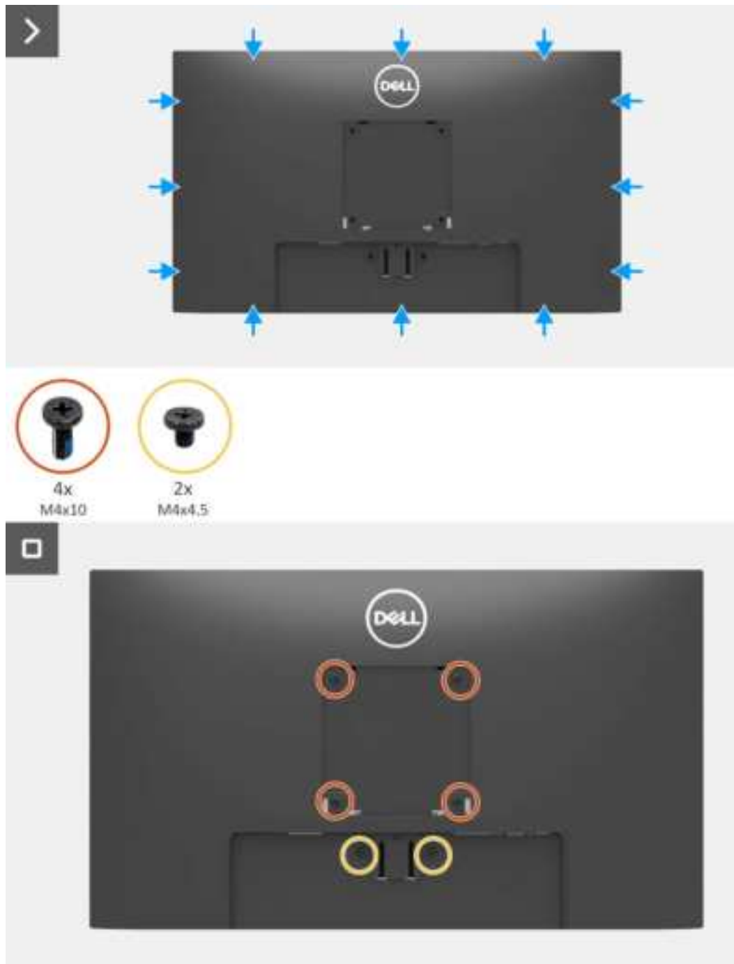
Figure 14. Installing the back cover
