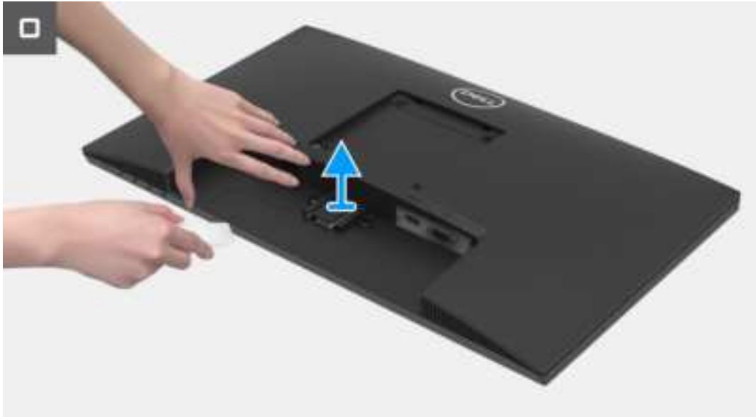
Figure 13. Removing the back cover
