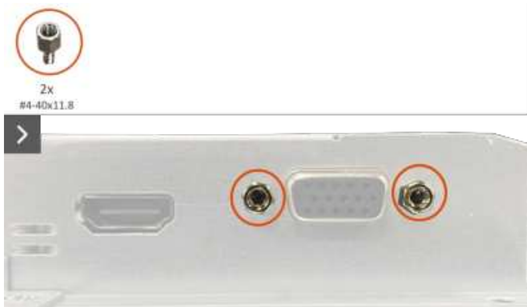
Figure 20. Removing the interface board
