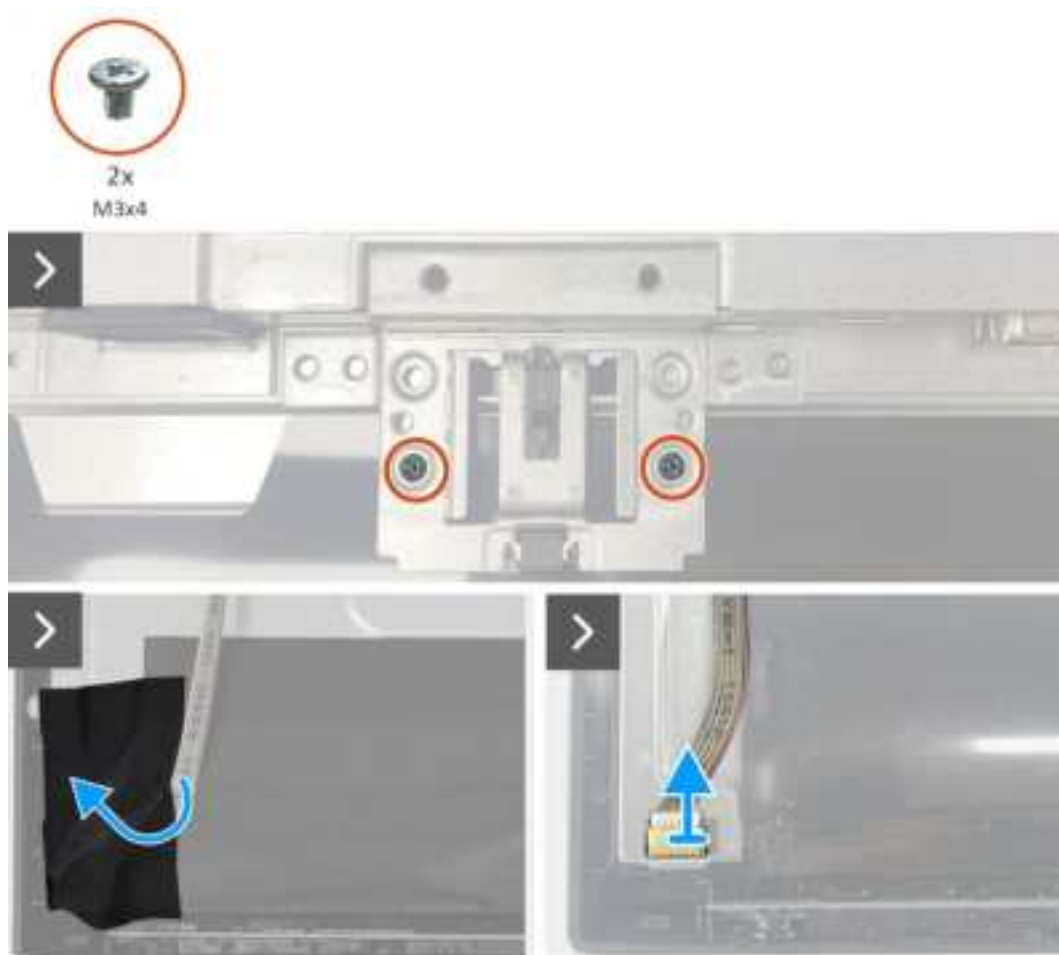
Figure 17. Removing the chassis assembly
