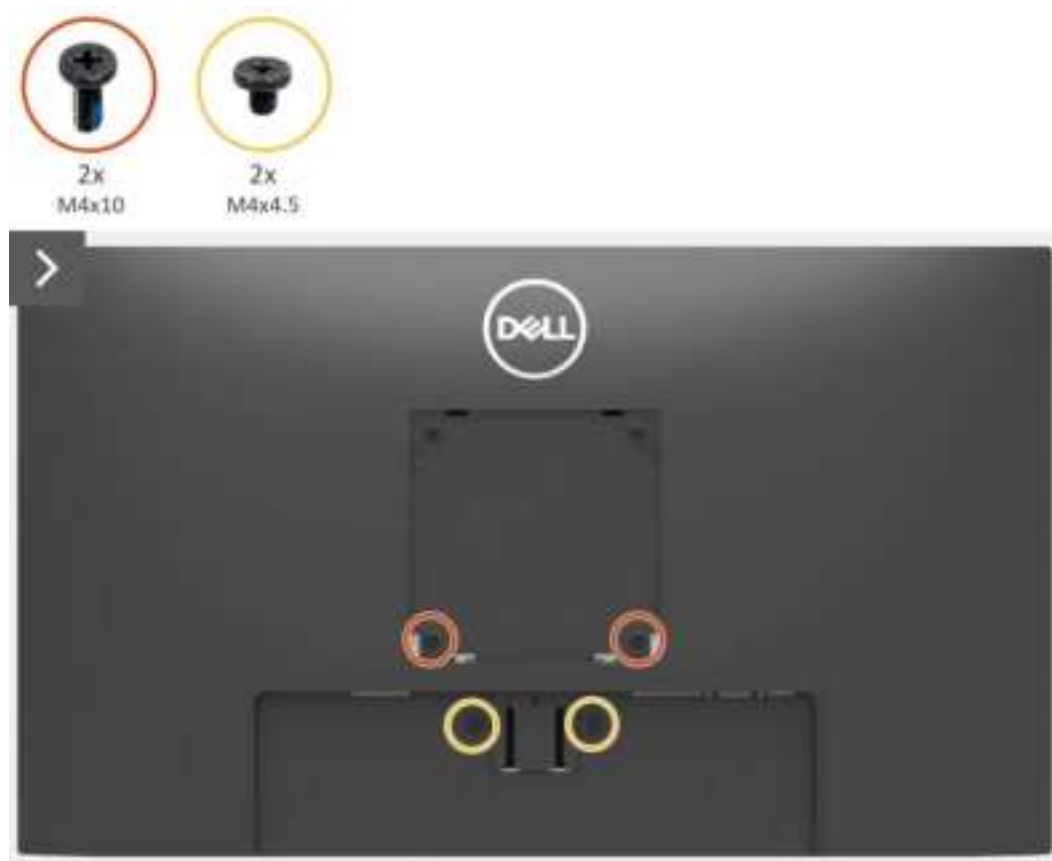
Figure 12. Removing the back cover
