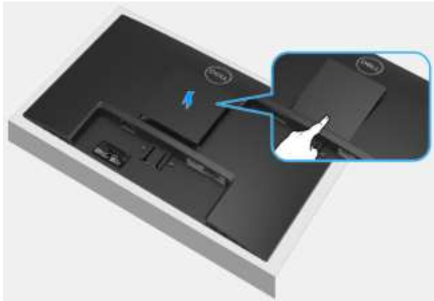
Figure 10. Removing the VESA cover
