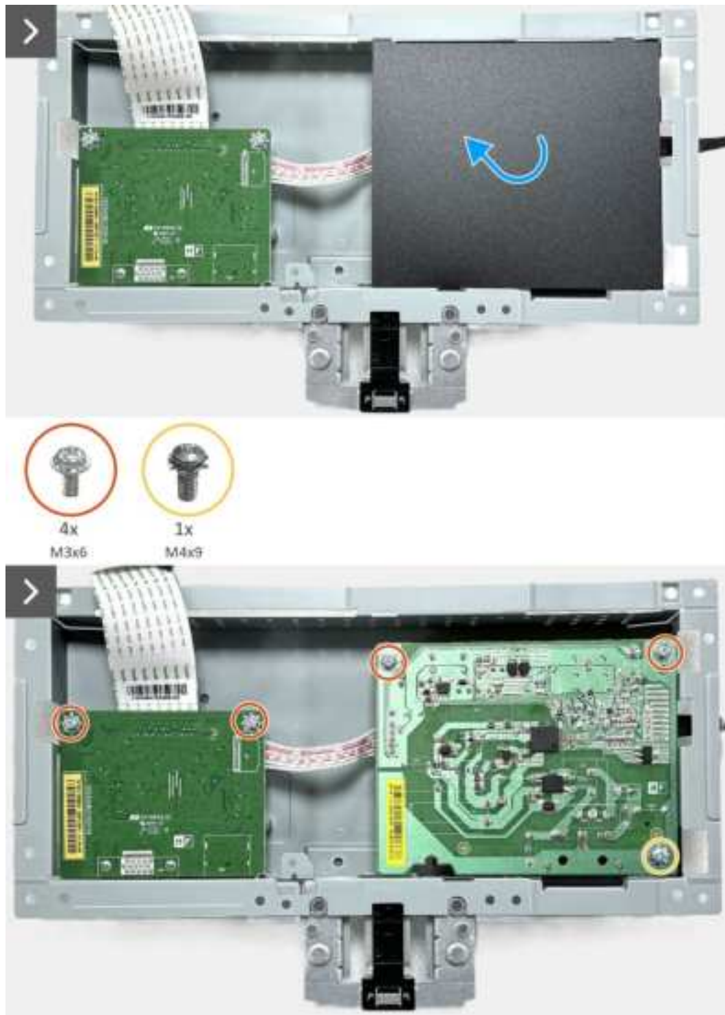
Figure 21. Removing the interface board
