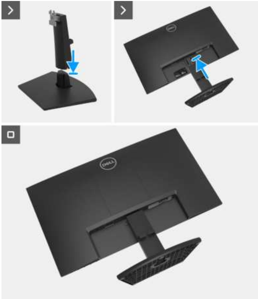
Figure 9. Installing the stand
