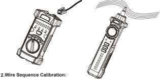
The wire sequence calibration is for the physical connection of the open, short, wrong, and reverse connection of the network line.
