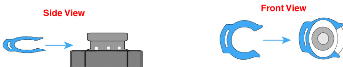
Fig.5 Install locking clips between the fitting body and ring/collet where applicable.
