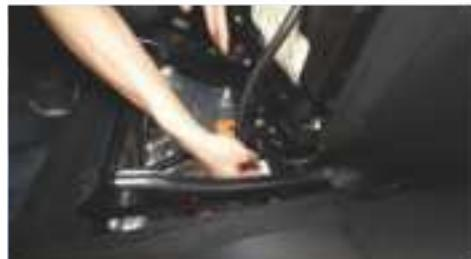
When lifting the back seat, pay particular attention to the fact that the seat has a power connection and that the connection has a plug. This plug can be loosened. It is advisable to loosen this plug before installing the seat cover in order to avoid tearing the wires. Of course, it is possible to install the cover without loosening the plug, but care must be taken to avoid tearing the power cable.
