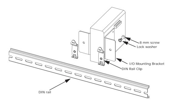
Figure 10.6: Mounting the Brackets on a DIN Rail
