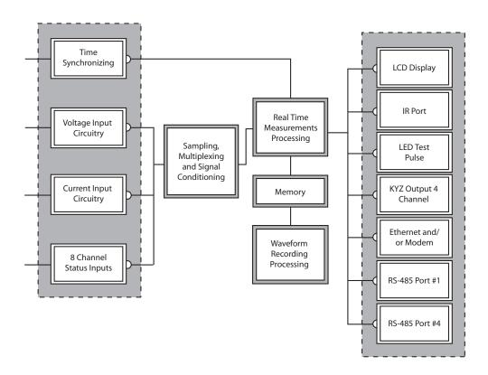
Figure 2.1: How the Nexus® 1262/1272 Meter Processes Inputs
