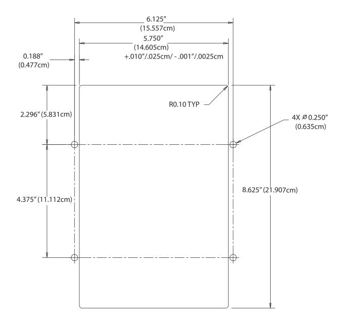
Figure 12.6: Switchboard Meter Cutout
