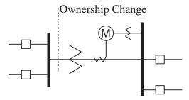
Figure 8.1: Low Voltage Metering Installation Requiring Loss Compensation
