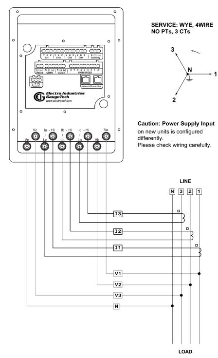
Figure 12.9: 9Z Transformer Rated Wye, no PTs, 3 CTs
