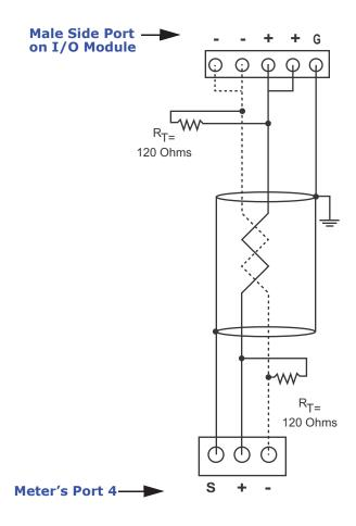
Figure 5.10: Meter and I/O Module Connections
