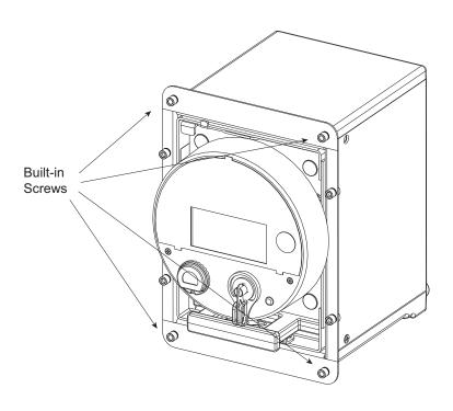
Figure 12.7: Switchboard Case Front Showing 4 Screw Holes
