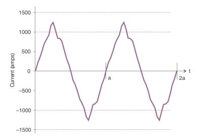
Figure 1.11: Distorted Current Waveform
