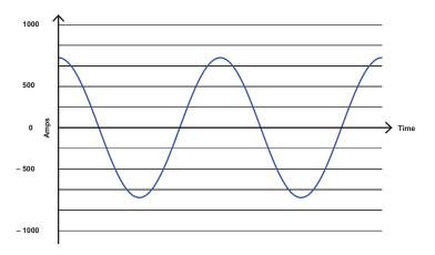
Figure 1.10: Nondistorted Current Waveform
