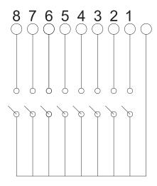
Figure 5.12: High Speed Inputs Connection
