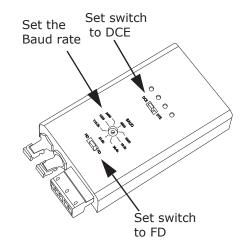
must match the Baud rate of the meter's RS485 port: you set the Baud rate by turning the screw to point at the rate you want.
