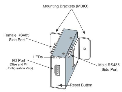
Figure 10.1: I/O Module Components
