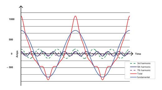
Figure 1.12: Waveforms of the Harmonics
