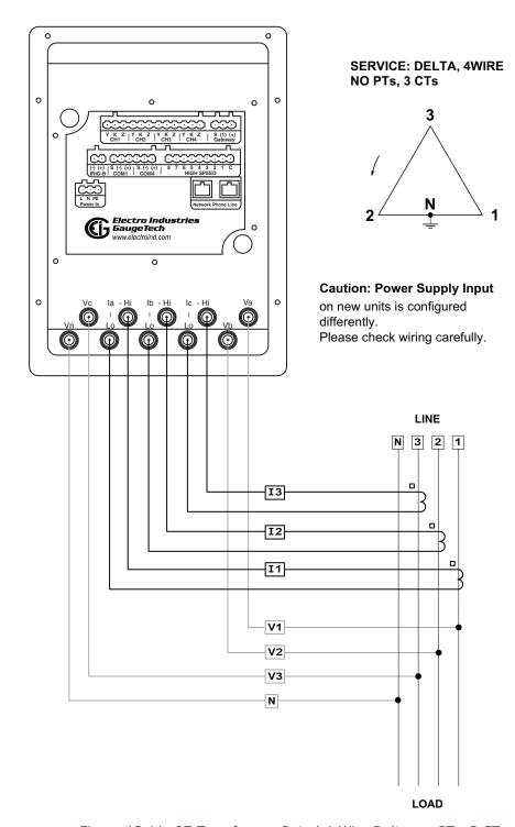
Figure 12.11: 9Z Transformer Rated 4-Wire Delta, no PTs, 3 CTs
