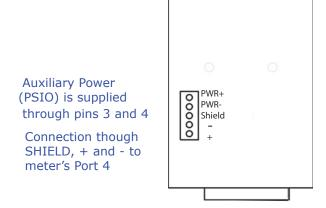
Figure 6.12: I/O Module Wiring Detail
