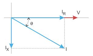
Figure 1.9: Voltage and Complex Current
