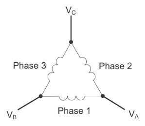
Figure 1.3: Three-phase Delta Winding Relationship
