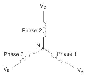
Figure 1.1: Three-phase Wye Winding
