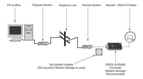
Figure 5.11: Remote RS485 Connections
