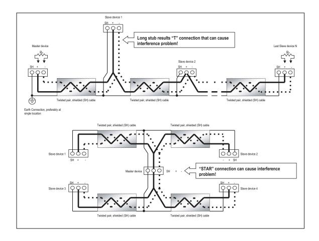
Figure 5.6: Incorrect "T' and "Star" Topologies
