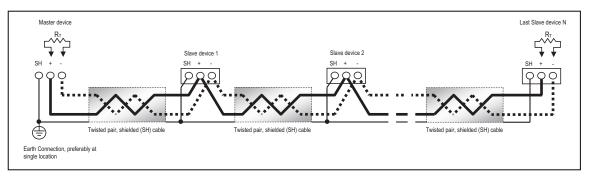
Figure 5.5: RS485 Daisy Chain Connection
