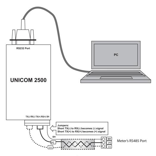
Figure 5.7: Meter Connected to a PC Using Unicom 2500
