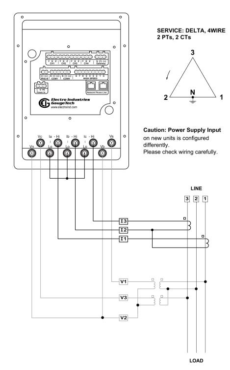
Figure 12.14: 9Z Transformer Rated 3-Wire Delta, 2 PTs, 2 CTs
