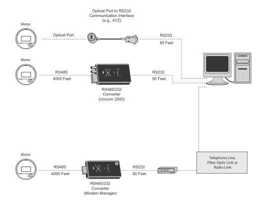
Figure 5.1: Serial Communication
