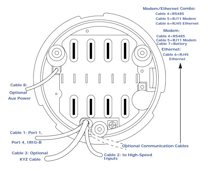
Figure 6.2: Socket Meter Rear View Showing Cables
