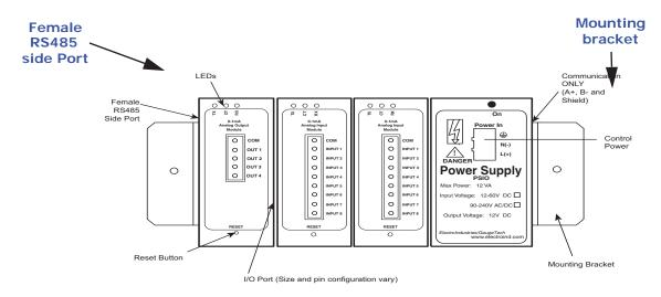
Figure 10.5: PSIO Used with Multiple I/O Modules
