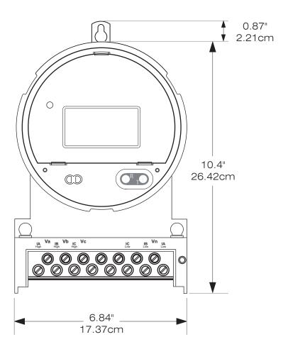
Figure 6.3: Socket Meter Mounted in A-Base Front View
