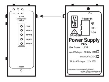
Figure 10.3: Power Flow from PSIO to I/O Module
