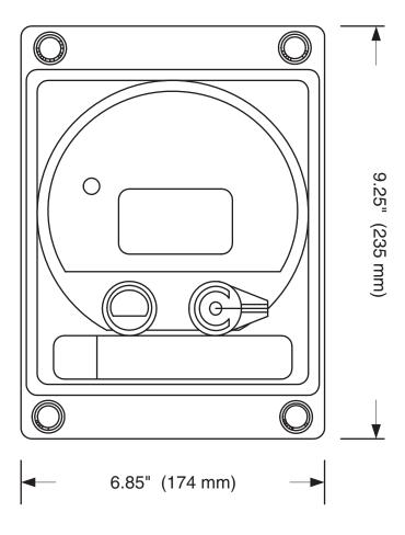
Figure 12.1: Switchboard Meter Dimensions, Front
