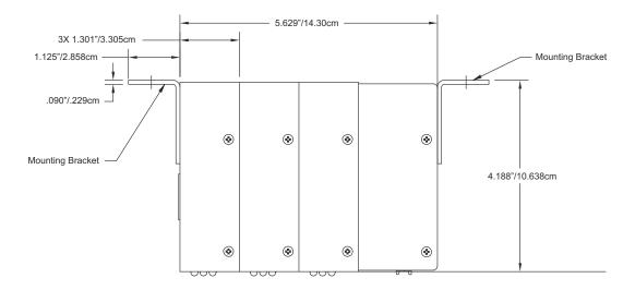
Figure 6.8: I/O Modules Mounting Diagram, Overhead View
