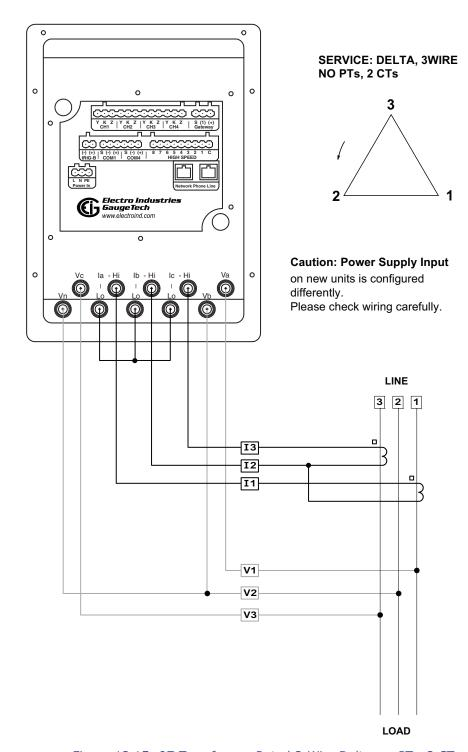
Figure 12.15: 9Z Transformer Rated 3-Wire Delta, no PTs, 2 CTs
