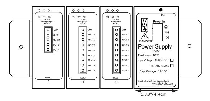
Figure 6.11: I/O Modules with PSIO Power Supply
