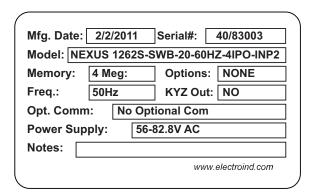
Figure 12.3: Sample of Switchboard Options Label
