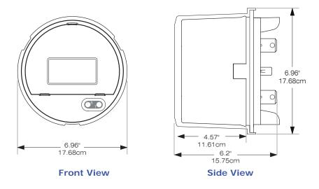
Figure 6.1: Socket Meter Mounting Dimensions
