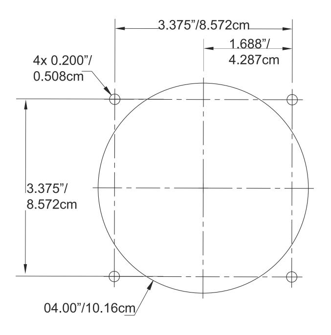
Figure 6.7: P40N/P40N+ ANSI Mounting
