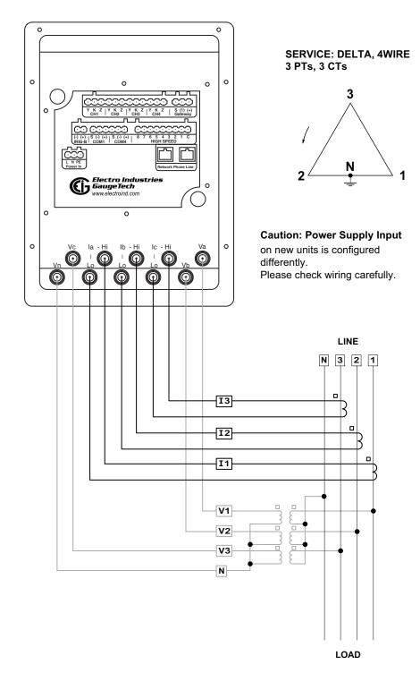
Figure 12.12: 9Z Transformer Rated 4-Wire Delta, 3 PTs, 3 CTs
