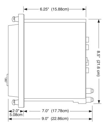
Figure 12.5: Switchboard Meter Dimensions, Side
