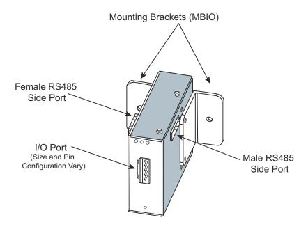
Figure 6.9: Single I/O Module with Mounting Brackets
