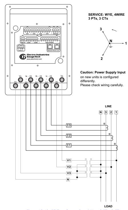
Figure 12.10: 9Z Transformer Rated Wye, 3 PTs, 3 CTs
