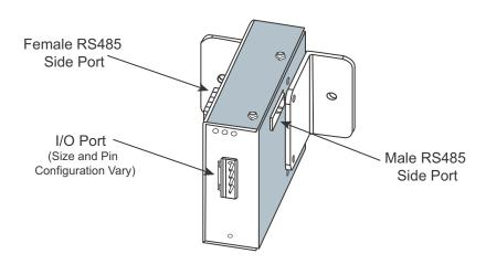
Figure 5.9: I/O Module Communication Ports
