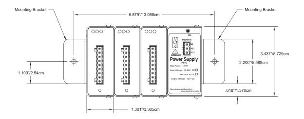
Figure 6.10: I/O Modules Mounting Dimensions, Front View
