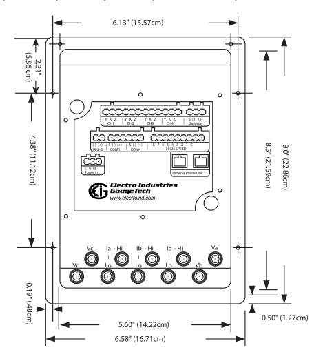
Figure 12.4: Switchboard Meter Dimensions, Back
