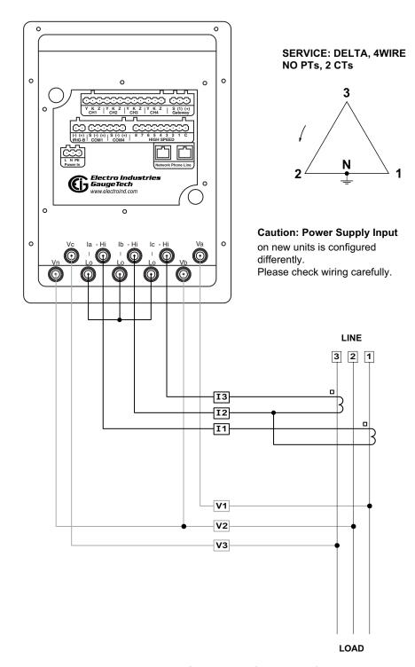
Figure 12.13: 9Z Transformer Rated 3-Wire Delta, no PTs, 2 CTs
