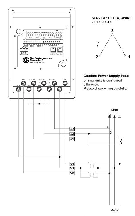
Figure 12.16: 9Z Transformer Rated 3-Wire Delta, 2 PTs, 2 CTs
