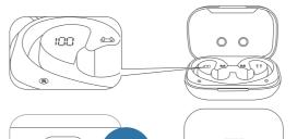
Note: The right display panel indicates the charging status per earbud. There are separated power consumption indicators by 4 grids in total, the indicator light will always flash during charging.
