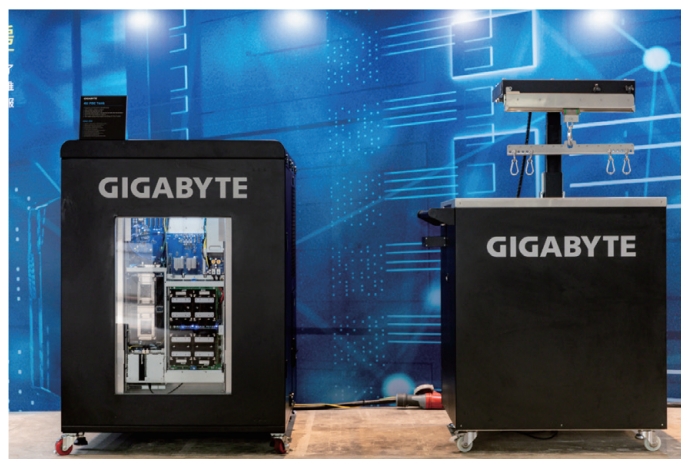
▲ 4U POC Tank & IT Lift
