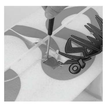
TIP: Plug a spare extension lead into the servo when removing to make it easier to route the lead of the replacement servo when installing it.
