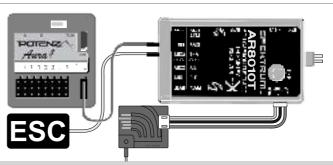
Note: When using Spektrum SRXL to connect to the Aura, always connect the remote receivers to the Spektrum receiver, NOT to the Aura.
