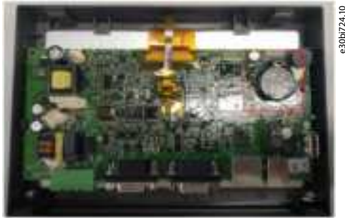
Illustration 87: Location of the Battery Inside the HMI
