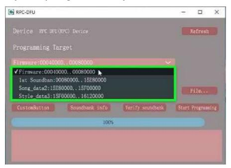
• Click File..., locate the firmware file (NPK20\_Soundbank\_20220517.bin), then click Start Programming. Wait until the status bar reaches 100%. Do NOT unplug the USB cable or power supply during this process.
