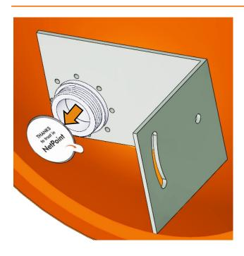
As a final step, remove the label that carries as a seal to avoid the entry of moisture or dirt into the waveguide.
