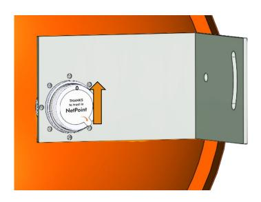
The mark made on the washer should be in the direction of the track on the plate, since that ensures that the spoke is in a correct position.
