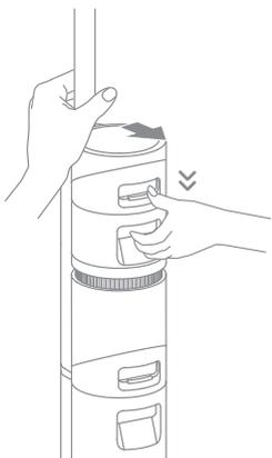
2. Open the tank cover and add enough clean water to the clean water tank.
