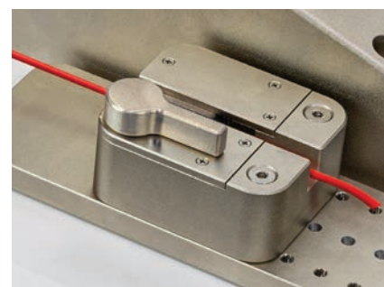
▲ The standard self-tightening wedge grip secures and pulls the loose end of the cable.
