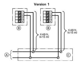
Two Vitotrol 200-E can be connected to the same control unit.
