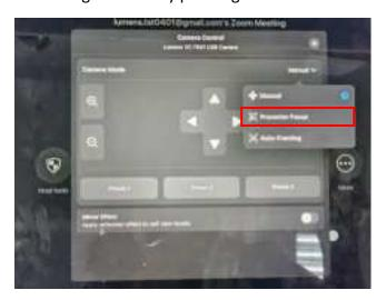
5. On the VC-TR41's webpage, there are different tracking modes available. The desired tracking mode should be selected beforehand, before pressing the Presenter Focus button on Room zoom controller.
