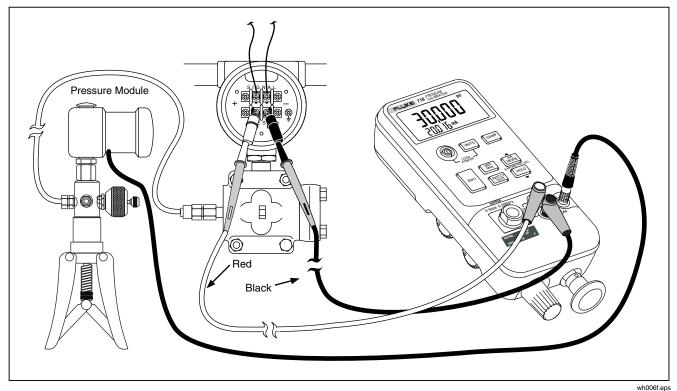
Figure 6. Pressure Module with External Pump
