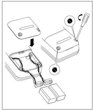
Figure 8. Battery Replacement
