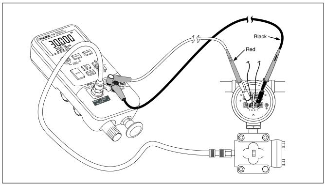
Figure 4. Internal Pressure Sensor with Internal Pump
