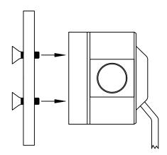
Once the sensor is mounted to its mounting plate, the sensor can be mounted to a wall, bulkhead or stringer. For proper operation, the sensor must be mounted where the fluid flow is horizontal and not vertical (Up and Down). The sensor also cannot be mounted flat (floor mounted) but instead must be mounted onto a vertical structure.
