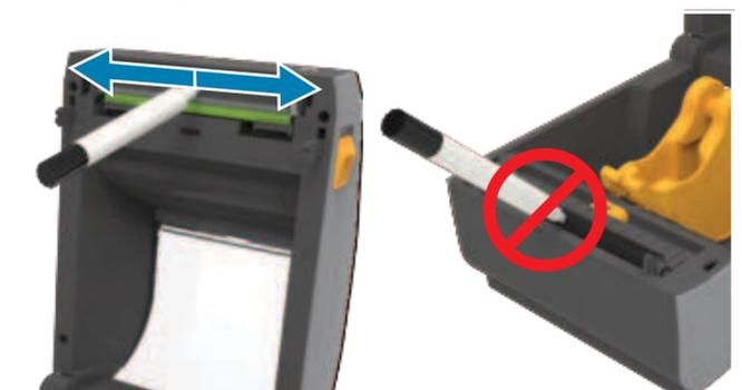
Clean printhead with a cleaning pen. Clean from the middle to the outside. Do not use a cleaning pen on the platen.
