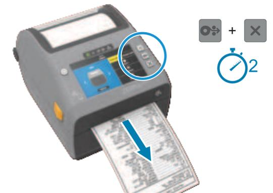
Press and hold the Feed and Cancel buttons for two seconds to print a configuration report.
