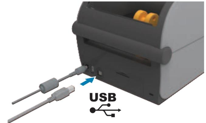
Connect a USB cable to the printer, connect the other end to your computer.
