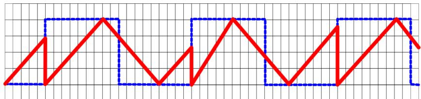
Triangle Wave Hard Sync'd to Pulse Wave
