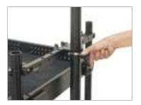
• Loosen the ratchet knob and open the clamp on the tripod holder bar.
