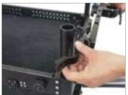
• Align the crossbar and secure it by tightening the side clamp knobs.
