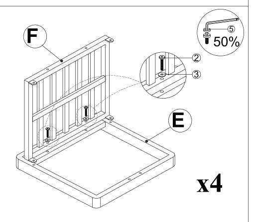
Connect Leg Stool (E) & Seat Stool Frame (F), Tighten Bolt (2) & Flat Washer (3) with Allen Key (5).
