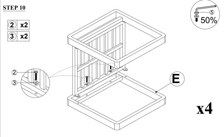
Connect the part from step 9 & Leg Stool (E) & Tighten Bolt (2) & Flat Washer (3) with Allen Key (5).
