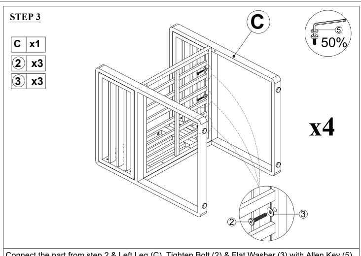
Connect the part from step 2 & Left Leg (C), Tighten Bolt (2) & Flat Washer (3) with Allen Key (5).
