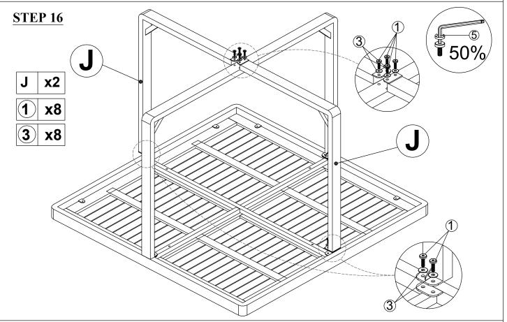
Connect the part from step 15 & Table Leg Left (J) tighten Bolt (1) & flat washer (3) with Allen Key (5).
