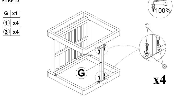
Connect the part from step 11 & Support stool (G) Tighten Bolt (1) & Flat Washer (3) with Allen Key (5).
