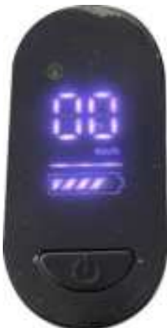
Mode 2: Green indicator Speed limited to 18km/h
