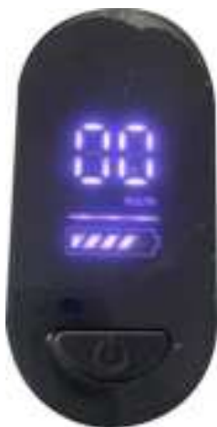
Mode 1: No indicator Speed limited to 6km/h
