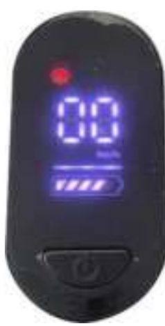
Mode 3: Red indicator Speed limited to 25km/h
