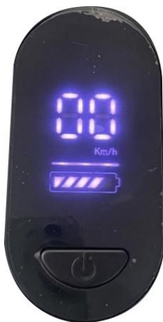
Mode 1: No indicator Speed limited to 6km/h
