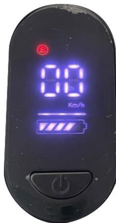
Mode 3: Red indicator Speed limited to 25km/h
