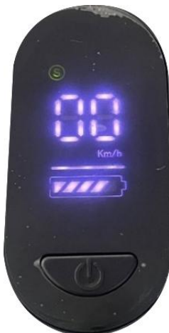
Mode 2: Green indicator Speed limited to 18km/h
