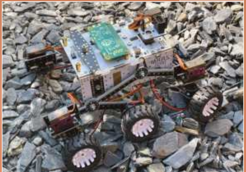
▼ A clever rocker-bogie suspension system enables M.A.R.S. Rover to clamber over large obstacles
