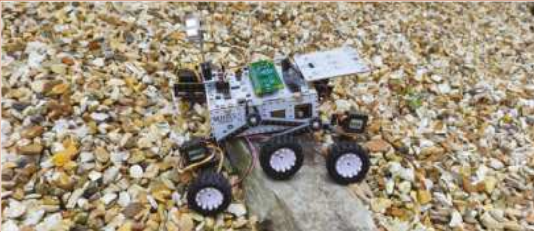
◀ The 4tronix M.A.R.S. Rover looks very much like the real thing and can handle tough terrain
