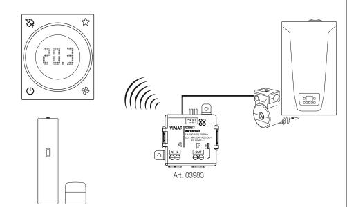
This type of application requires the presence of at least one magnetic contact 03980 and module 03983.
