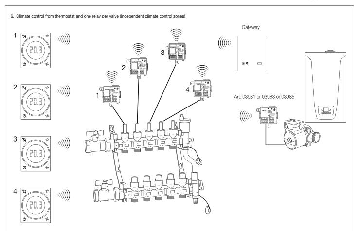
This type of application can either be "Summer" or "Winter" and the thermostat should be set with its output configured as a remote relay; use one of either art. 03981, 03983 or 03985 configured as a remote actuator for "consent to boiler/circulation pump" to control the valves.
