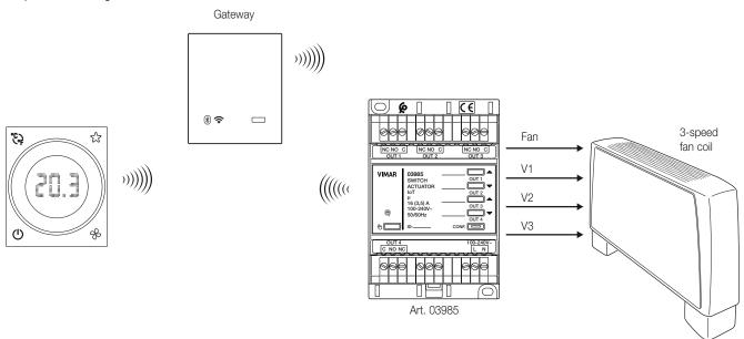
This type of application can either be "Summer" or "Winter" and the thermostat should be set with its output configured as a 3-speed fan coil; use actuator 03985 to control the fan coil. In the View Wireless App, create the Climate Control group  $\rightarrow$  Remote relays and Heads  $\rightarrow$  Summer/Winter  $\rightarrow$  3-speed fan coil
