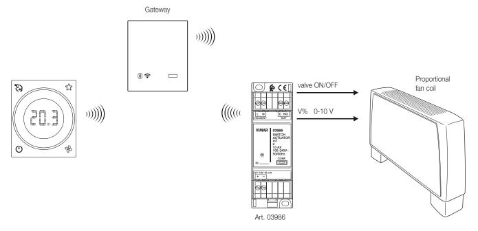
This type of application can either be "Summer" or "Winter" and the thermostat should be set with its output configured as a proportional fan coil; use actuator 03986 to control the fan coil. In the View Wireless App, create the Climate Control group - Remote relays and Heads - Summer/Winter - proportional fan coil
