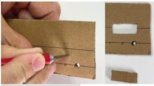
Once you've finished tracing around the pickups, you can remove them from the template.
