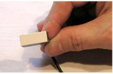
Trim the excess adhesive from the pickup on all sides, using a sharp pair of scissors, so you end up with the tape aligned with the edges of the pickups.
