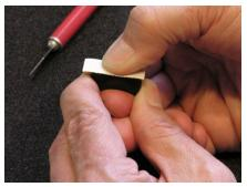
Apply a strip of the included temporary white adhesive to the red sensing surface of each of the pickups. Using your thumb, press the adhesive over the entire red sensing surface of the pickup to bond it.
