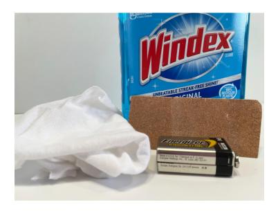
Wipe the bridgeplate clean with a clean cloth <u>lightly</u> moistened with water or Windex™, and allow it to dry for at least 10 minutes. NEVER use Naptha™, lighter fluid or any other cleaners like this to clean the bridgeplate or pickup, as these will leave deposits behind that will destroy any chance of obtaining a proper bond. Pure Acetone can be used to remove any stubborn adhesive left behind, but use it sparingly, and don't get it on the finish of your instrument.
