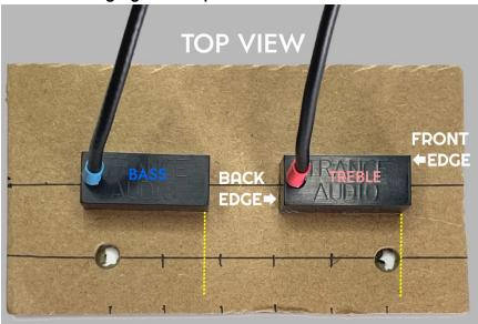
The front edge of the treble (red) side pickup is lined up to the far edge of the hole for the high E string.
