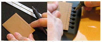
Using the ruler, draw a line about ½" inside along one edge. Then place the template centered next to the bridgepin holes. Mark the position of each of the holes along the edge of the template and on the line.
