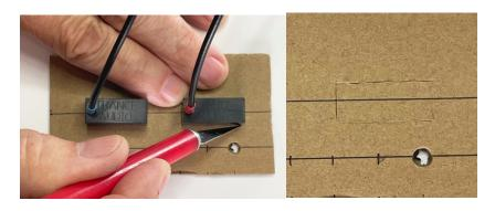
Once you've got the pickups placed correctly, use the X-Acto knife to score the cardboard as close as possible around the pickups. The idea here is to create a cutout in the cardboard that will hold both pickups securely in place while you transfer the template to the inside of the guitar and install it in the proper place at the bridgeplate. Using the X-Acto knife to trace closely around the pickups will allow you to create a template to easily do that.
