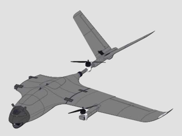
Now insert the wings and route all the cables from the motor and servo to the channel in the wing that leads to the fuselage. Repeat the same process with the second wing.
