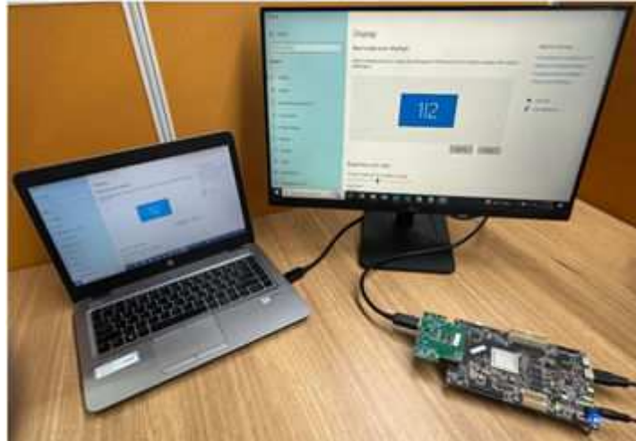
Figure 3-2. HDMI TX Displaying the Laptop Data from DisplayPort Rx
