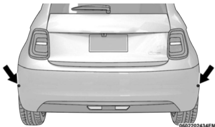
Radar Sensors Location
