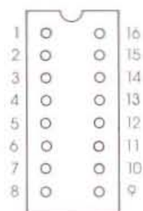
Figure D-8 Internal game connector pin-outs
