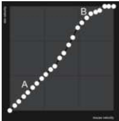
**(A) Increasing Thrust for Aiming / (B) Prevent High Turn Speed**
