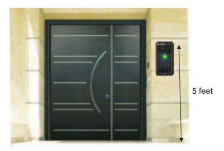
The recommended installation height for the camera is 5 feet above the ground.
