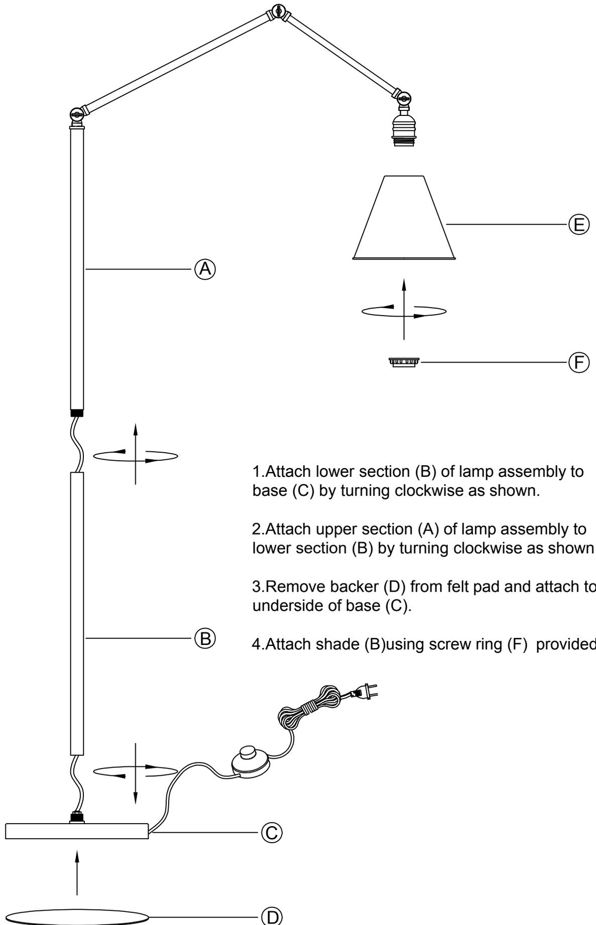
1. Attach lower section (B) of lamp assembly to base (C) by turning clockwise as shown.
